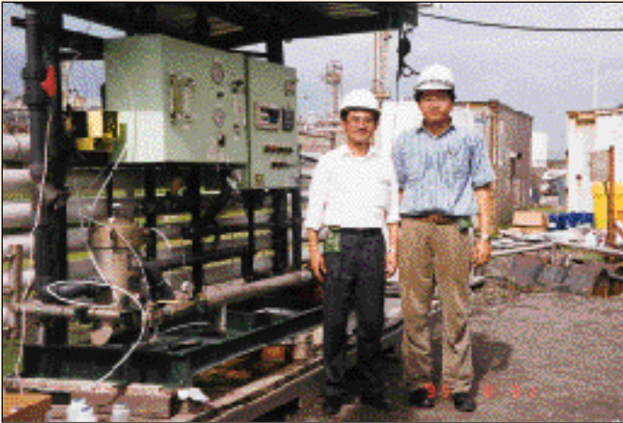
Brown and Caldwell engineer Joe Wong and J. A. Kuo of Enprotech System Corp. used an innovative, membrane-based (ultrafiltration/reverse osmosis), 25-gallon-per-minute pilot treatment system to test industrial wastewater reclamation at a major petrochemical plant in Taiwan.
